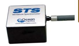
STS takes advantage of recent advances in CMOS detectors that elevate optoelectronic performance and improve system reproducibility. It uses a 1024-element ELIS-1024 linear image sensor that's responsive from 200-1100 nm and has excellent sensitivity (6.74V/lux-second typical). This new generation of CMOS detectors offers excellent performance with great value.
